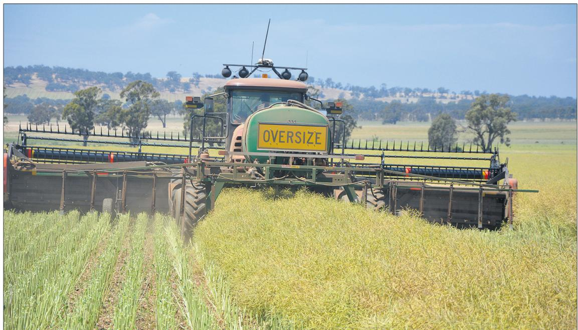
**Forward planning . . .** A Goldacres sprayer is hooked on behind to spray rye-grass in preparation for next year's crop; the swather front also sprays the chemical on either side of the windrower.
